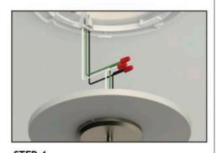
STEP 4 Plug it in and twist to lock new light into place!
