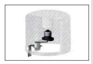
STEP 2 Remove your light bulb and screw in Quick Connect™ socket adapter
