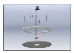
STEP 1 Attach Ceiling Ring™ with screws around your recessed light
